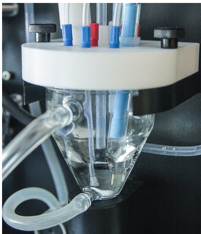
Image: close-up of the analysis vessel inside the wet part of the TitrLyzer®.
